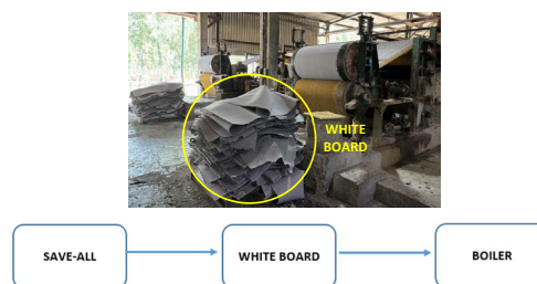
Fig. 4: White board sludge recovery for use in boiler
