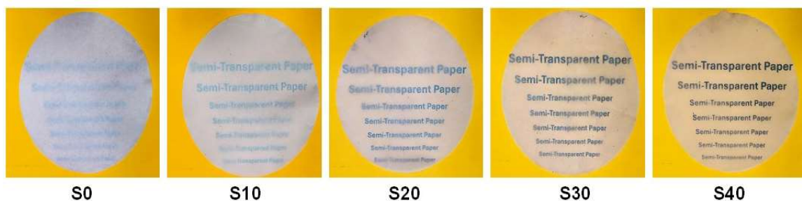
Fig 3: Effect of concentration on optical transparency of developed semi-transparent papers
