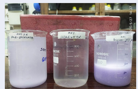
Figure 7: MPS Inlet feed, outlet clarified water & underflow recovery (from L to R).
