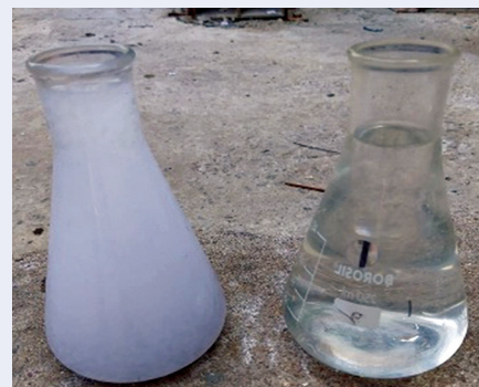
Figure 3: MPS Inlet feed and outlet clarified water (from L to R).
