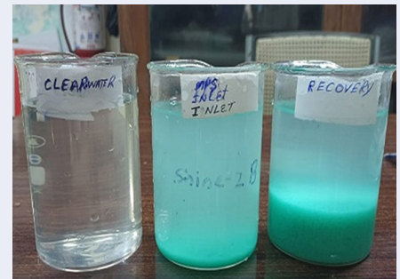
Figure 8: MPS outlet clarified water, Inlet feed water and underflow recovery (from L to R).
