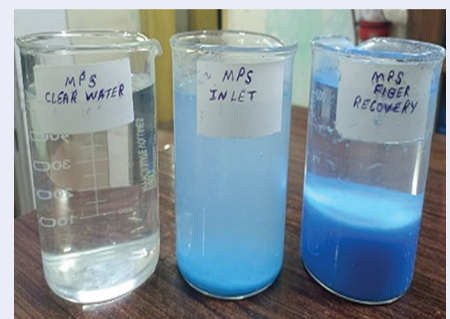
Figure 9: MPS outlet clarified water, Inlet feed water and underflow recovery (from L to R).
