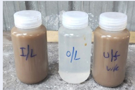
Figure 6: MPS inlet feed, outlet clarified water and underflow sludge (from L to R).
