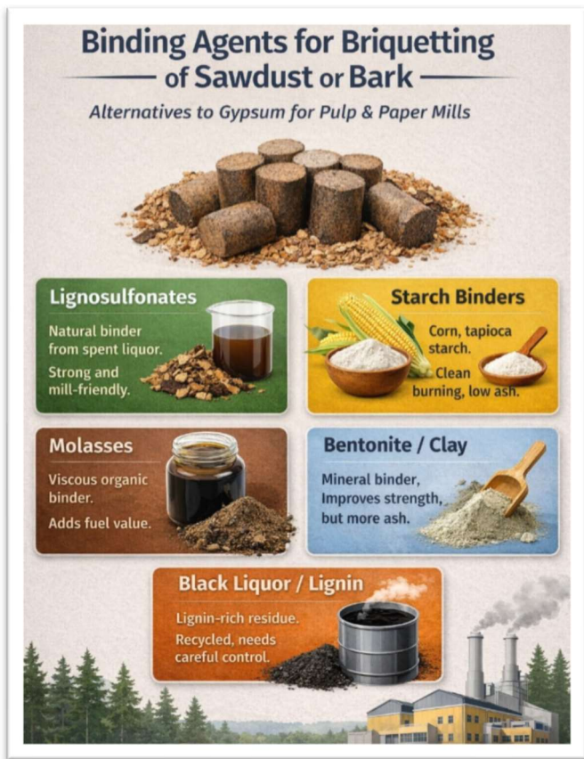
Fig 1. Different technically viable binders for briquetting sawdust or bark
