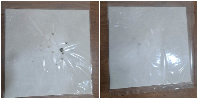
Images 9 & 10: Impact of fire on firewall (top and bottom sides)
