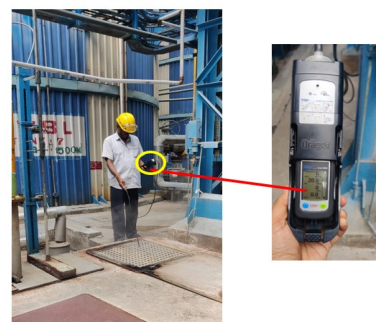
Fig. 10: LEL measuring at NCG drain area
