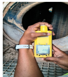
Fig. 7: LEL measuring in confined space
