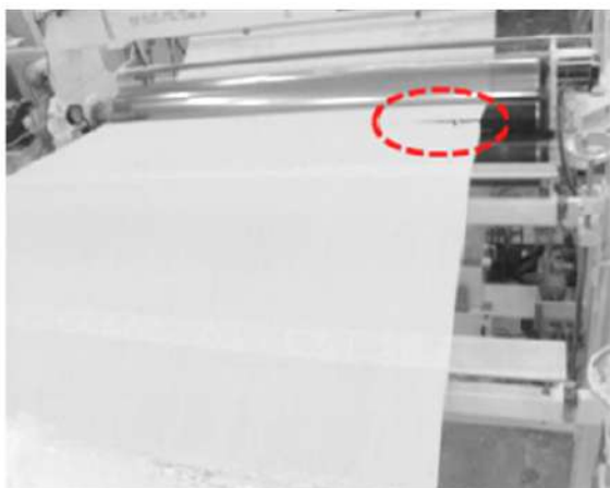
Figure 15: Shows a hole (left image), most likely generated on the tissue machine, causing a break on the infeed for the converting line (right image).
