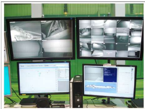
Figure 7: Shows how a fully integrated, single platform, web monitoring (WMS) and web inspection (WIS) operator station that allows a defect to be automatically from the WIS to be transferred to the WMS system synchronized to the same piece of paper: This allows for a rapid and accurate means for the user to find the source of the defect and to eliminate it. A single keyboard and mouse is able to operate both systems.
