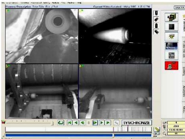
Figure 14: Tissue and towel converting is a new application area for WMS. Recent installations have demonstrated significant efficiency improvements in eliminating breaks and identifying their sources. The above shows, with 4 cameras, how the toilet paper log production is interrupted due to system not inserting the core in time.
