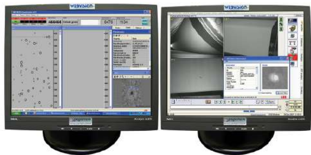
Figure 16: Example of a combined WIS (left) and WMS (right) operator control station display set-up providing total visibility to all of the machine cameras synchronized to the same piece of paper. Full two-way software integration provides automatic image transfer via pop-ups, as well as defect classification information, and other important variables to help speed up solving the root cause.
