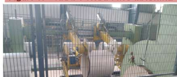
Figure 10 – KRAFT WRAPPING MACHINE
