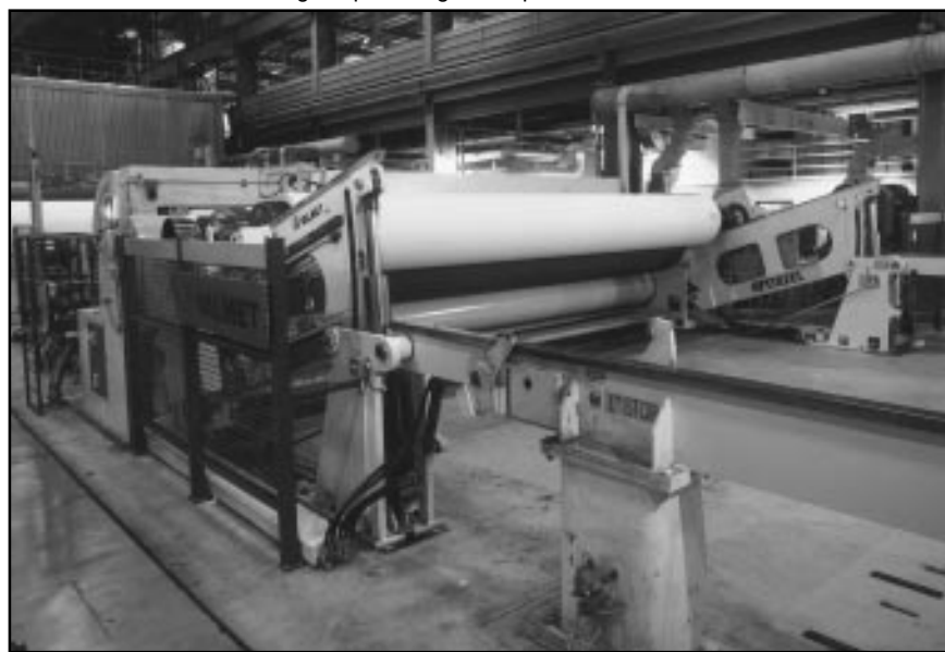
10. Blandin Paper Co., Grand Rapids, MI, operates a rereeler with rails which can be raised and lowered for variable-angle nip loading of the parent reel
