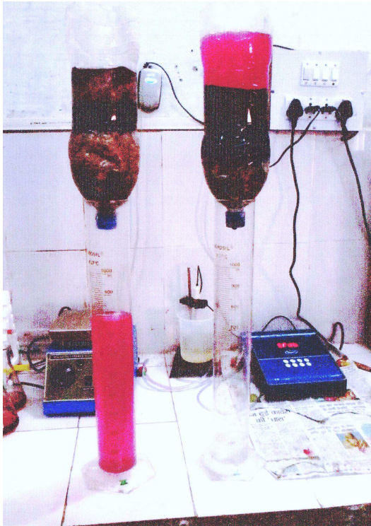
Image 2: Filtration in progress. Left: Activated Carbon; Right: Pet coke fly ash
