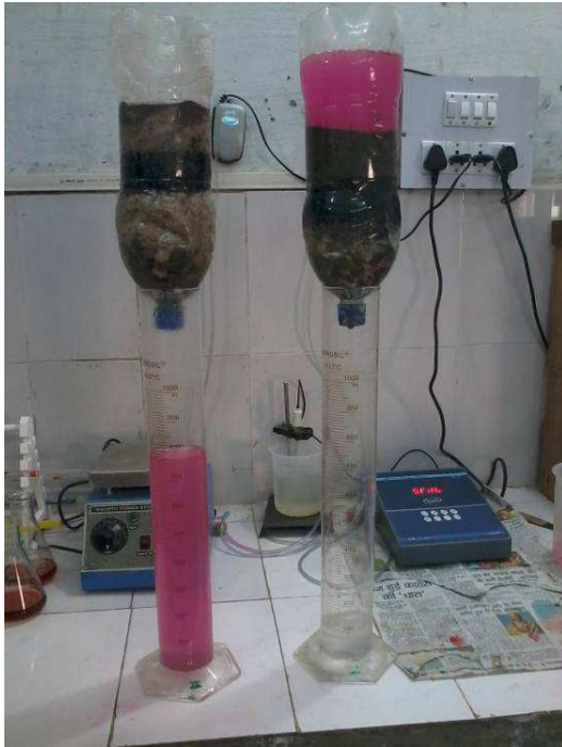
Image 2: Filtration in progress. Left: Activated Carbon; Right: Pet coke fly ash
