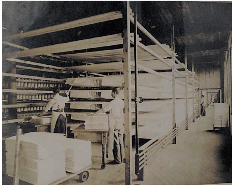
Fig. 7.26 Loft drying in a Western hand paper mill. Damp sheets are hung in gatherings or spurs on ropes extending across the loft.
