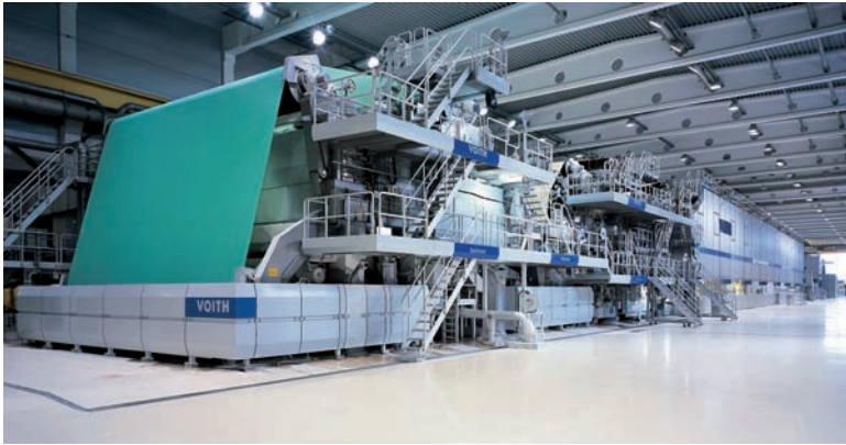
Fig. 7.1 View of a modern papermaking machine used to make newsprint.
