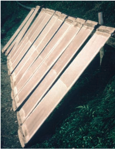
Fig. 7.27 Drying single sheets of hand-made paper in Japan. Damp sheets are brushed into contact with boards that are exposed to sun to accelerate the drying process.
