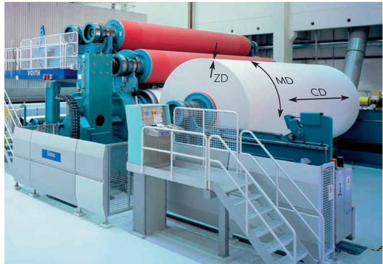
Fig. 7.4 An image of paper on a paper machine illustrating the three perpendicular directions. Machine direction (MD) is aligned parallel with the movement of the web through the paper machine. Cross machine direction (CD) is aligned parallel to the wind-up reel. The zed direction (ZD) is parallel to the thickness direction of the web. It is perpendicular to the principal plane of the web formed by the MD and CD vectors.
