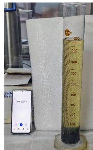
Fig 14: Clarification of Agro-based EOP Filtrate through Electro-coagulation
