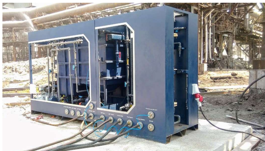
Fig 15: Efficacy of treatment of ETP water with Electro-coagulation & Specialized Ultrafiltration
