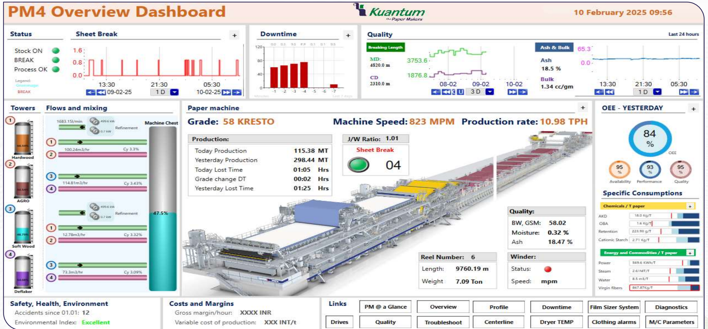
PM-4 Overview - Integrates live process data with visuals, providing a real-time operation view
