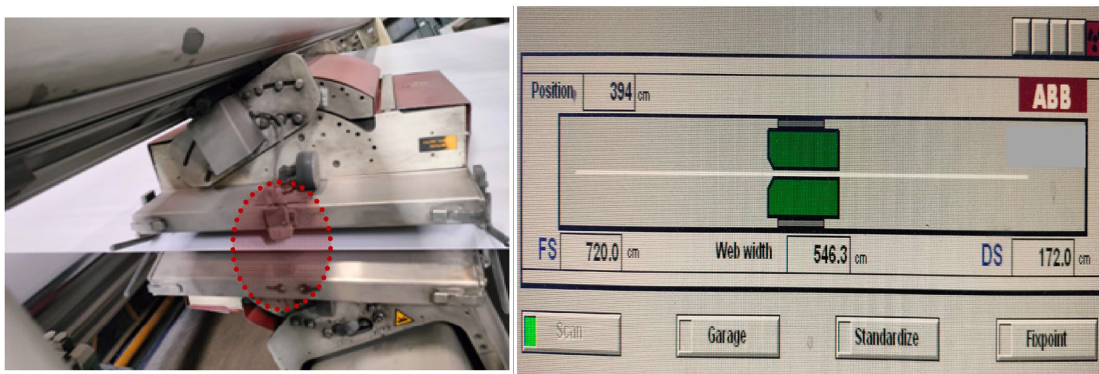
Figure: 1 Auto Edge OFF Sheet Sensor in Scanner & Sheet Width display in DCS Graphics
