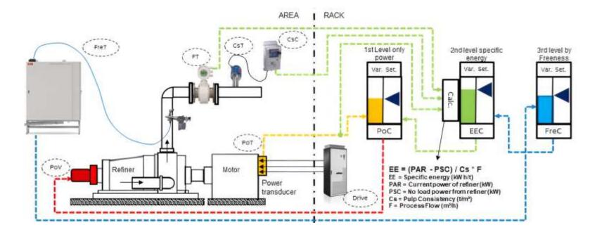
Before Online Freeness measurement was installed, it would take the mill up to six hours to achieve uniform paper production during grade change to meet the required specs. Now it takes less than an hour
