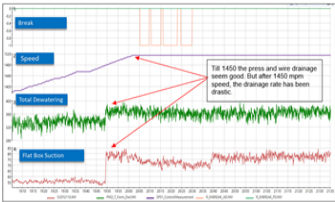
Figure 11 – Break detected due to drainage
