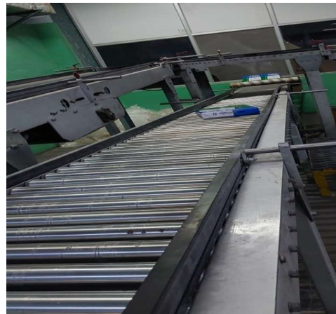
Fig 24. Before Integration- Single Reams getting discharged
