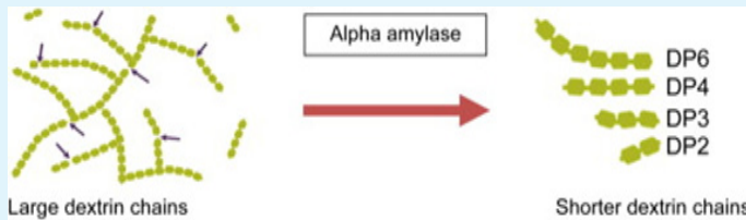
Fig. 5 Amylase activity on dextran molecules present in Corrugation gum and breakdown to smaller segments [4]
