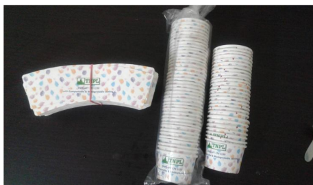
Fig 2: Blanks and cups made with PLA coated board
