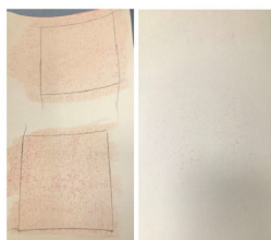
Fig 4: Pinholes in barrier layer
