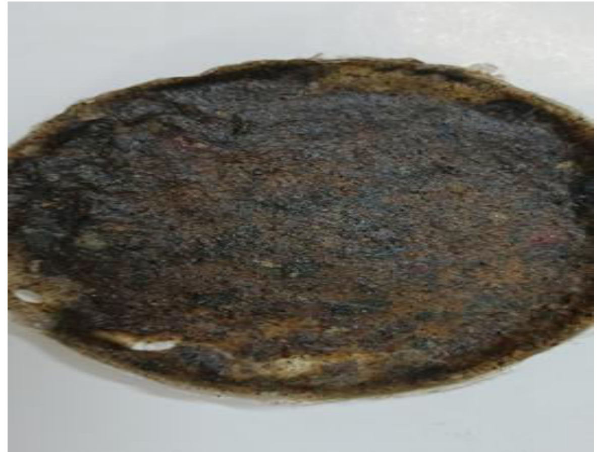
D: Dried bioplastic film without filtration
