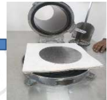
e) Now, transfer the sheet with placing bloating paper over the fresh sheet
