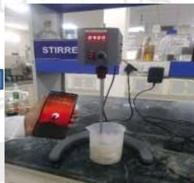
g) Now, Stir the mixture with mechanical stirrer with the speed of 900rpm for 30 min.
