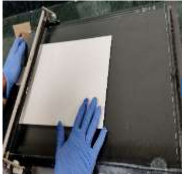
a) Placing sheet on the AFA
