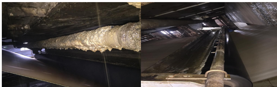
Fig. 10: Slime formation on the machine parts (Left- Before trial, Right- After trial)
