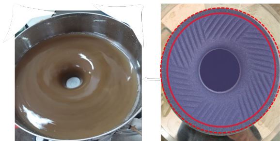
Fig. 1. Vortex formation during refining of nanocellulose at Zero clearance (left). Stationary upper grinder with grinding zone of 17 mm width (gap between solid and dotted circles) (right)
