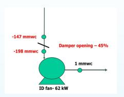
the system requirements. Avoiding the damper loss by installing VFD for the fan results in significant energy savings. As indicated in the following case study, the pressure drop across the fan inlet damper was 51 mmWc which was equivalent to 25% of the fan head. Installing VFD and opening the damper fully or removing the damper will result in a saving 25 kW in fan power. The power reduction will be as per the affinity law where power  $\alpha$  speed3.
