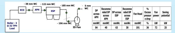
The pressure drop across ESP was 63 mmWc is also on the higher side as compared to the norms of 30 mmWc. This can be due to turbulence at ESP inlet duct and bends in the duct. The excess pressure drop in the above case was 36% of the fan head. Significant energy-saving potential exists in the boiler ID fan by reducing the pressure drop by checking the condition of the APH
