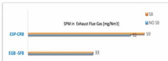
Fig -19 : Comparison of SPM in exhaust flue gas [mg/Nm3] -During Soot blowing & No Soot blowing in CRB [with ESP] &SFB [with EGB]
