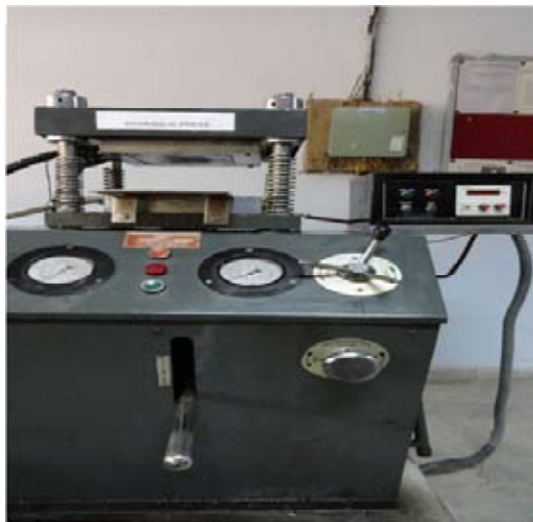
Fig. 1: Hydraulic compression moulding machine
