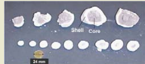
Figure 5- Cross Section of nodules from a lime Kiln (3)
