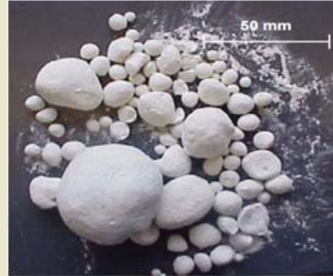
Figure 4- Nodules larger than 25 mm have a dark, uncalcined grey core, surrounded by a white calcined shell (3)
