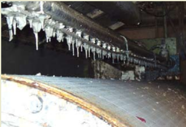
Figure 1. Stringers caused by Filamentous bacteria
