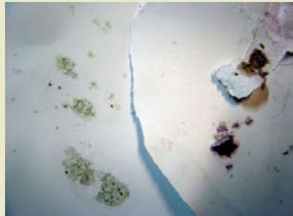
Figure 2. Slime spots in finish paper / board. Changed to purple color with slime test reagent
