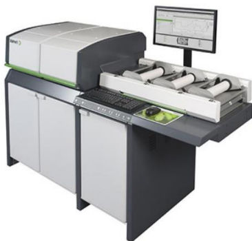
Figure 5 – Automated board and paper testing system
