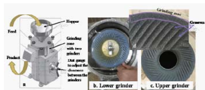
Fig 2: Super Masscolloider set up, (b). Lower rotating grinder with leftover slurry, (c). Upper stationary grinder, (d). Grooves for smooth flow of slurry and the actual grinding zone in a Super Masscolloider.
