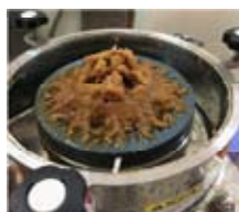
Fig 4:Deposition or piling-up of micro cellulose fibres on the lower rotating grinder at 0.3 units of clearance due to the high consistency of pulp (8.33 g/L). This piling-up was not observed when consistency of pulp reduced to 3.12 g/L.
