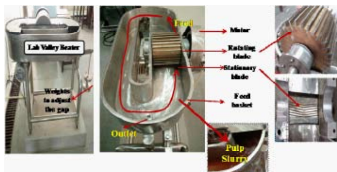
Fig 1: Lab Valley Beater. Front view (left), top view (middle) and beater plate-stationary and beater roll-rotating.
