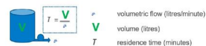
Figure 2. Residence time of a vessel equals its volume over its discharge flow
