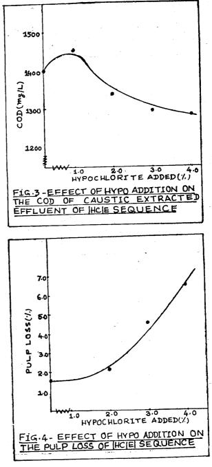
residual lignin content of HC/E/ Pulp. The optimum hypo was about 2% considering the total chlorine consumption and cost of chemicals, quality of pulp, pulp loss and pollution load compared to C/E/H sequence.
