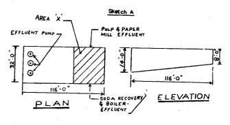
Within a week after mill started operating its effluent treatment plant, it was observed that the area marked 'X' in the *Sketch A* got filled up with settled solids, rendering that portion of the sump quite ineffective for retention. Hence it was decided to modify the Central collection sump as per *Sketch B* given below, thus reducing the retention time in the sump to about 6 minutes:
