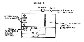
Along with this modification care was taken to ensure that the velocity of entry of the effluent into the sump does not exceed 1 ft. per second, as this approach velocity avoids turbulence near the affluent pumps. As can be seen from *Sketch B*, intermediate baffle walls had also to be constructed between the effluent pumps as a precaution against vortex formation, which affects the efficiency of pumping.
