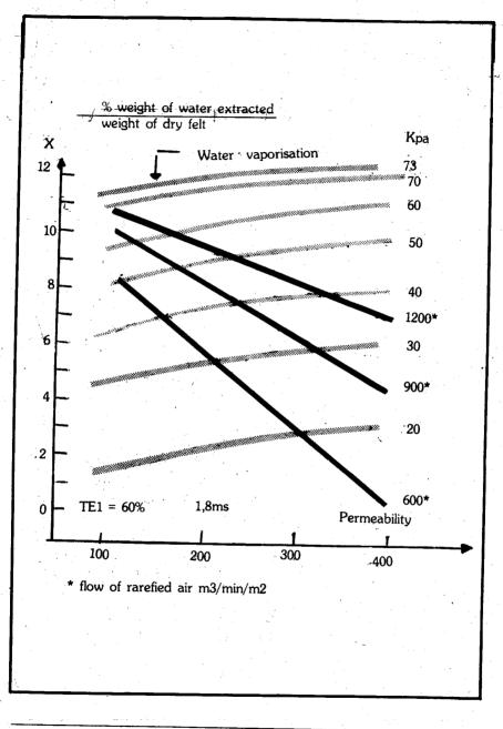
The choice of the vacuum source is based on the common behaviour of the felts and illustrates the necessity of maintaining high permeability-porosity during their aging.
