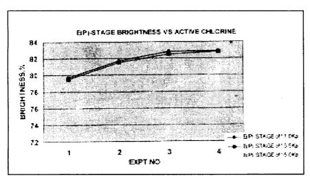
brightness losses (6). Lower Kappa numbers achieved from Extraction stage after D<sub>1</sub> stage will produce a much stable, high bright, high strength pulp with less colour reversion.
