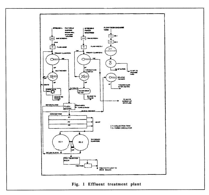
clarification into the coloured effluent primary clarifier, whenever CSRMP was stopped. Though this gave some relief, the desired results could not be achieved. Hence the bagasse yard effluent is totally recycled.
