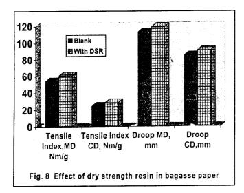
Machine. If the droop values are lesds, curling or bowling occurs as the moisture is driven out from the paper on heating. This results in heavy jamming inside the Machine. The dimensional stability of bagasse paper is low when compared to other wood papers for reasons already discussed. In order to improve the performance of the Bagasse paper another approach is now discussed. Increasing the bonding also strength results in better dimensional stability.
