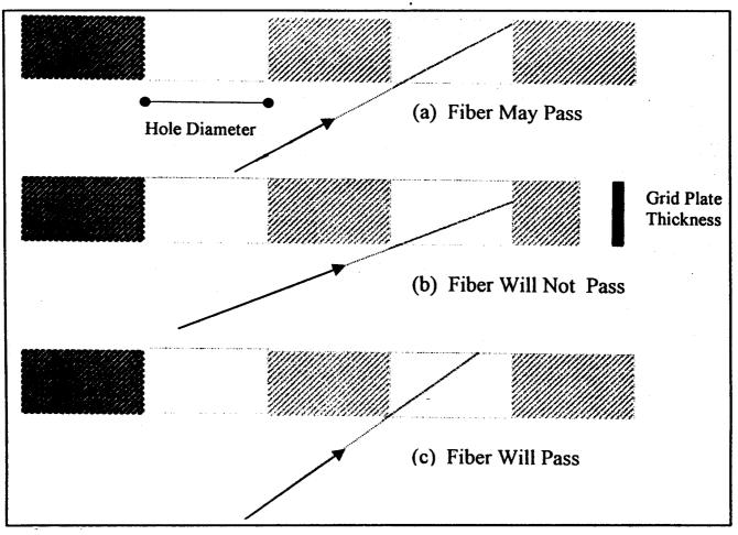
Fig. 1 : Cross Section View of Grid to Show Angle of Approach of Fiber & Possibility to Pass Through Grid Holes
