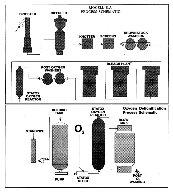
ADMT. The detailed design conditions are presented in the Table. The mill decided to purchase a white liquor oxidation (WLO) system as a source of alkali for the StatOx medium consistency oxygen delignification. The Oxypro<sup>TM</sup> WLO system has not only a very high sulfide efficiency conversion and low operating costs, but is also environmentally friendly.
