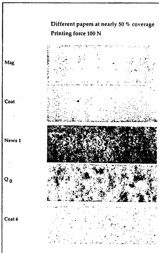
Figure-6 Typical prints on different grades of paper
