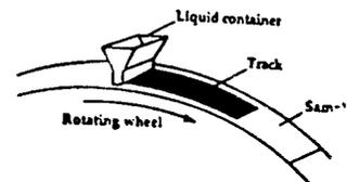
Figure-8 The Bristow absorption tester (Bristow<sup>23</sup>)
