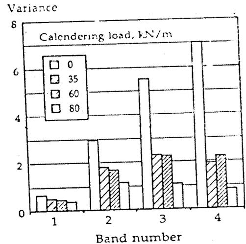
Figure-12 Effect of calendering on the variance of the profile in the four wavelength bands
