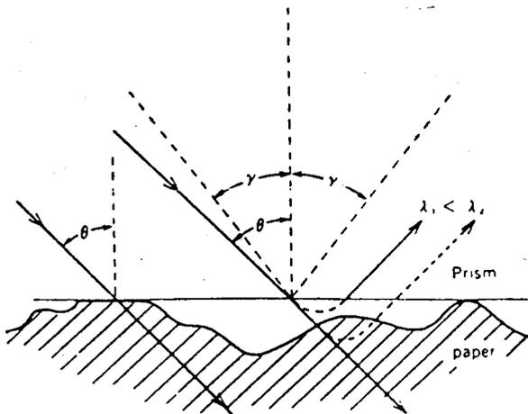
Figure-5 Effect of wavelength of light in discriminating contact and non-contact areas
