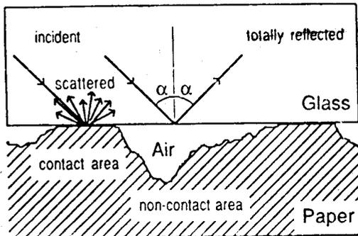
Figure-4 Light distribution at contact and non-contact areas in the FOGRA tester
