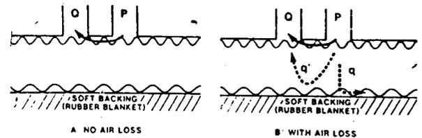
Figure-3 Schematic diagram of the PPS tester showing the possibility of error due to leakage of air through the bulk of the sheet (Mangin and DeGrace<sup>2</sup>)
