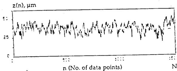
Figure-9 A typical surface profile
