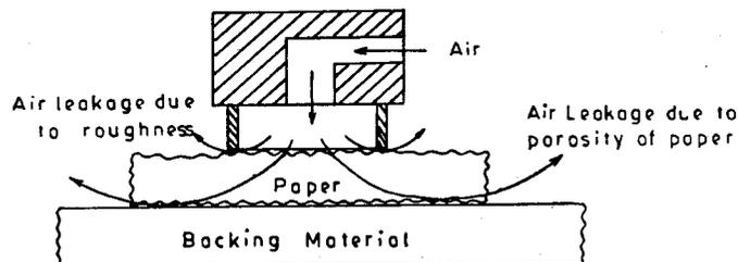
Figure-2 Air-leak method of roughness measurement
