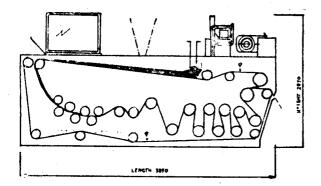
The above belt filter press is our basic machine and has all the features necessary to give good results. Here are some of the features :
