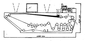
What distinguishes an HP press from a HP-F press is the extended drainage zone. The HP-F press is preferable when the hydraulic loading is high in relation to the dry content loading.
