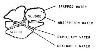
Different types of water in the sludge. Drainable water is found in the higher voids and can be removed by gravity. In the smaller units we find the capillary water held in place by capillary forces.
