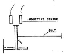
A spring loaded metal paddle rests against the edge of the cloth When the cloth is running properly in the machine this edge-sensor is exactly midway between two inductive indicators.
