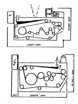
With a sludge to be dewatered and only moderate demands on outgoing dry content belt filter presses of types MP and CP are best.
