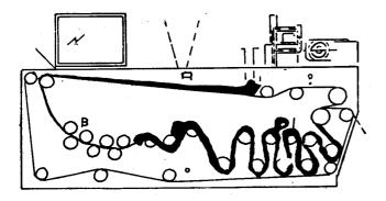
After zone A in the drainage stage the sludge should be so dry that the pressing forces in zone B do not press the sludge out sideways. The pressing/ shearing forces in zone C are higher and therefore demand a higher dry content. The dewatering is then finished off by increasing shearing forces in zone D. Shearing forces are regulated by the pressure on the c adle and these increase the greater the wrap round the press rolls and the higher the filter cloth tension.
