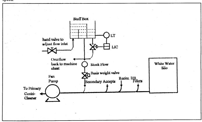
The basis weight valve should be located 2 to 3 metres below the silo level.
