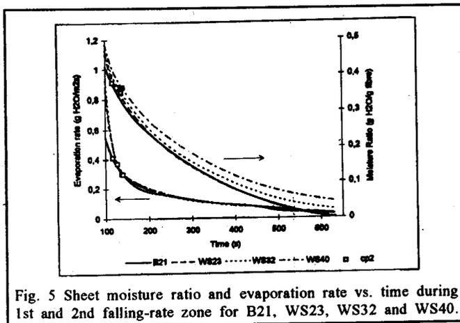
Fig. 5 Sheet moisture ratio and evaporation rate vs. time during 1st and 2nd falling-rate zone for B21, WS23, WS32 and WS40.
