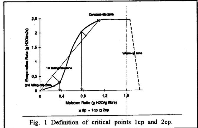
Fig. 1 Definition of critical points 1cp and 2cp.
