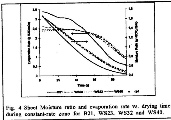
Fig. 4 Sheet Moisture ratio and evaporation rate vs. drying time during constant-rate zone for B21, WS23, WS32 and WS40.
