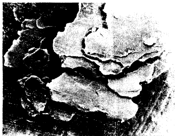
Fig.-1 : SEM micrograph of clay showing layering structure (X100)
