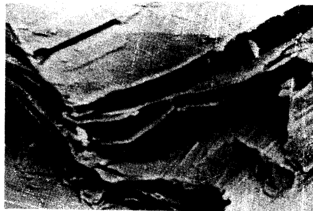
Fig.-2 : SEM micrograph of clay showing layering structure (X100)
