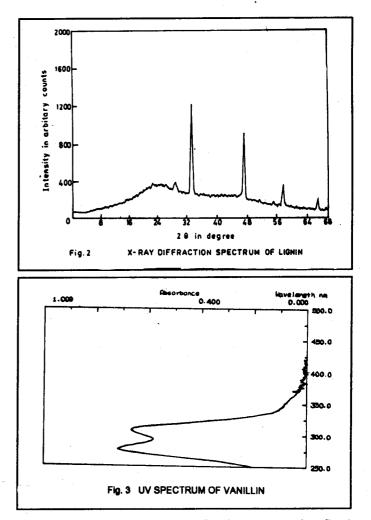
temperature controlled muffle furnace. The final temperature of the furnace was maintained for 2 hours. The ash content of lignin was found to be 0.3%. Similary the vanillin sample was also tested by chemical methods and instrumental method. The ultraviolet absorption spectra carried out by Jasco Model UV/VIS spectrophotometer 7800 using 1-cm cells in the regions 250 to 500 nm with methanol solution is shown in Fig. 3.
