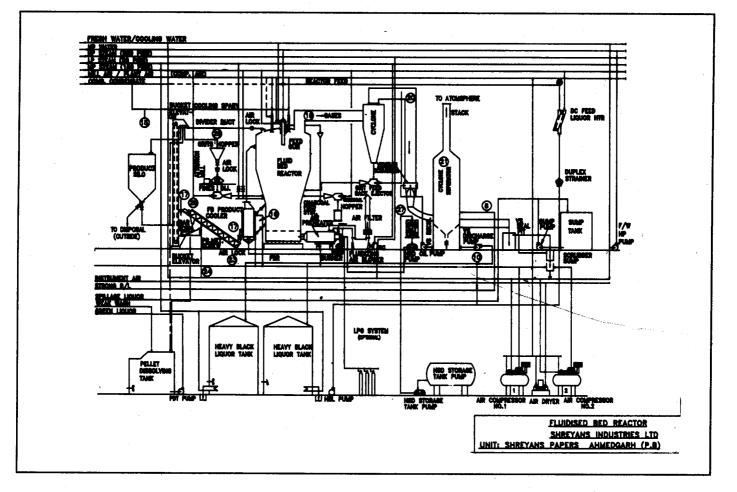
Arrangements has been provided to spray water or weak black liquor to bring down the temperature of the Reactor while auxiliary fuel like Charcoal or furnace oil can be used to increase the temperature.
