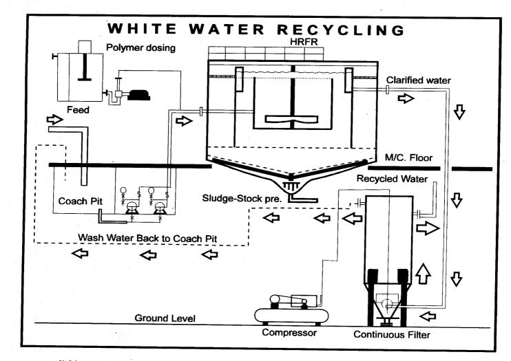
as a polishing unit after the clarifier which is capable of handling the fluctuations to deliver the consistent quality. Fluctuations in the inlet load condition will affect the performance of flotation saveall since the balance between suspended solids/ chemicals/ air dispersing ratio is very important and is very difficult to maintain.
