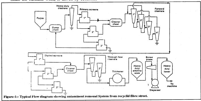
system from recycled fiber stock preparation street which will allow paper makers to control potential problems with recycled fiber more effectively.
