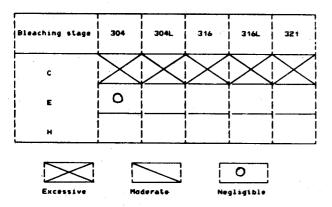
pitting and crevice corrosion (Tables 3-5) that the gaseous phase of C- washer is highly corrosive as compared to those
